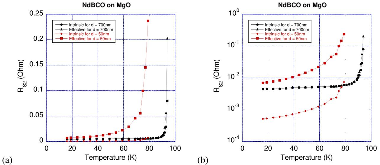
Fig. 11 Computed Surface resistance from  $\sigma$ : (a) linear scale (b) logarithmic scale
