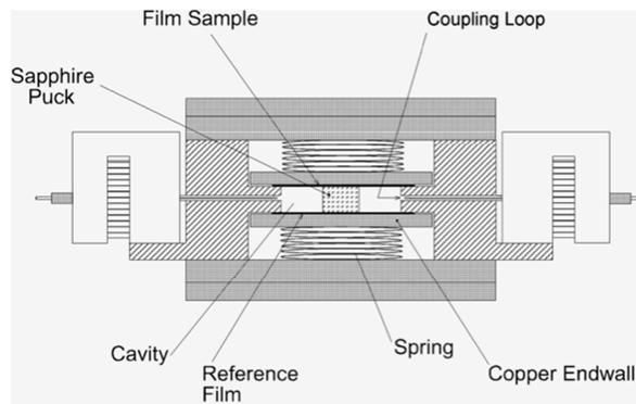
Fig. 1 Schematic diagram of Hakki-Coleman test resonator
