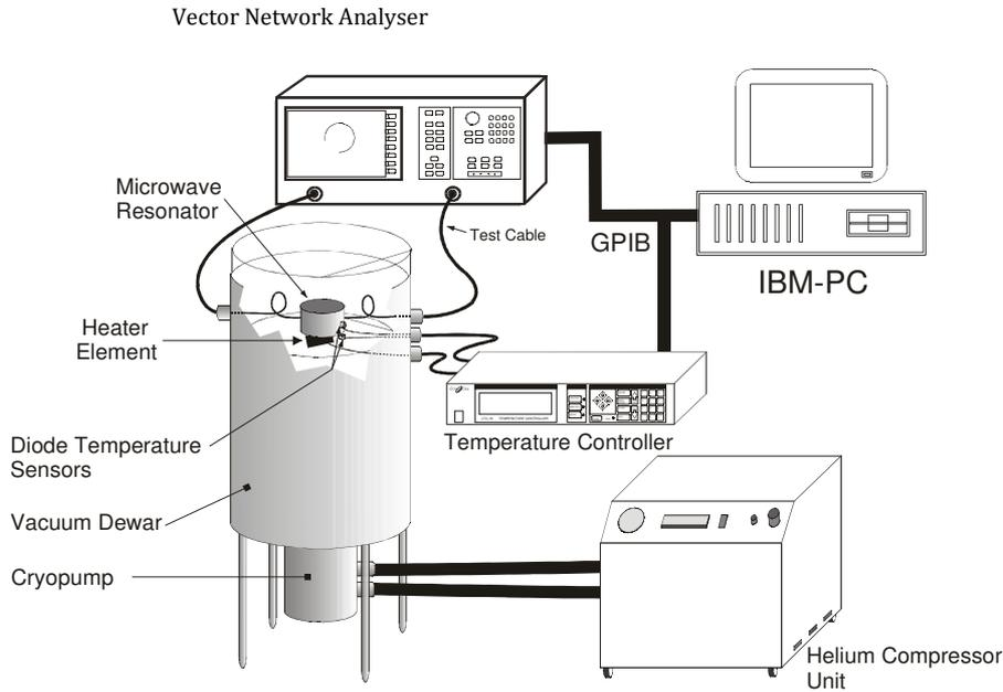
Fig. 6 Microwave characterization system
