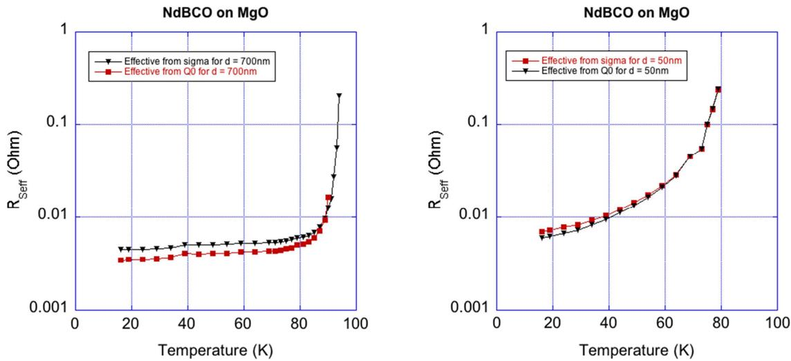
Fig. 12 Effective Surface resistance obtained from two approaches for (a) 700/800nm films and X170112B films, (b) for 50nm films
