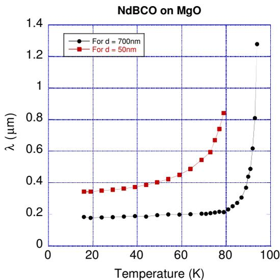
Fig. 9 Penetration depth from  $f_{res}$
